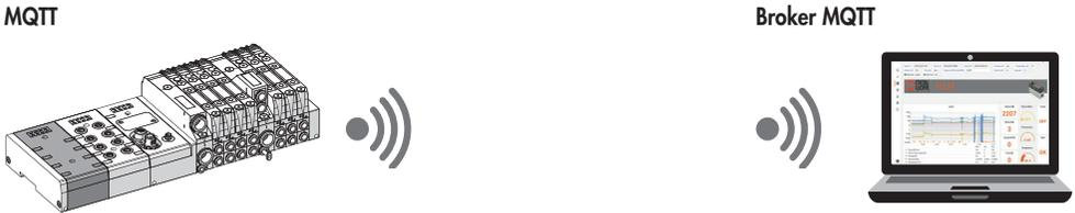
Gathering data from the field makes it possible to carry out a predictive diagnosis of the system; monitor the operating parameters at all times and optimize the operation of the machines and the pneumatic system. The software can be implemented with analysis functions that provide machine efficiency monitoring.
