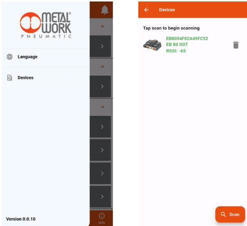
Press the **Scan** button to start searching for new devices. The devices recognised will be displayed in green. The RSSI value indicates the signal strength.
