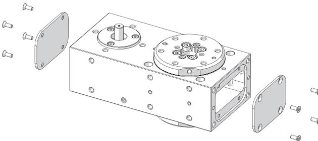
3. Remove the rotary flange by loosening the 4 screws that secure it to the driven pulley. This operation must be carried out twice in case of version with double rotary flange.
