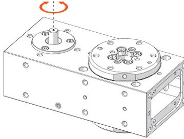
11. Tighten the grub screw applying the tightening torque indicated below to secure the position of the tensioner.
