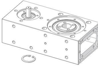
5. Assembly the bearing-retaining flanges to the motor side and tighten the screws securing them to the actuator body applying the tightening torque shown in the table. It is recommended to apply threadlocker like Loctite 243.
