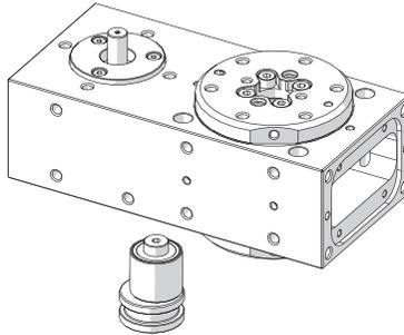
8. Apply threadlocker like Loctite 243 on the tensioner locking grub screw and screw it until it stops, go back 1 turn.
