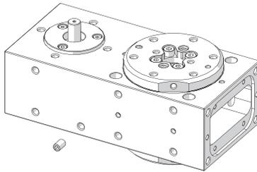
9. Rotate the tensioner clockwise towards (+) with a torque wrench applying the torque value indicated below. Maintain this torque and simultaneously rotate the rotating flange, first in one direction and then in the other, for a complete turn. This generates uniform tension on the belt along its entire path. The tension is in the correct range when the tensioner notch is close to the end of the arch corresponding to the (+) symbol.
