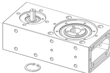
9. Pull out the pinion assembly.
