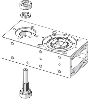
10. Pull out the driven pulley assembly.
