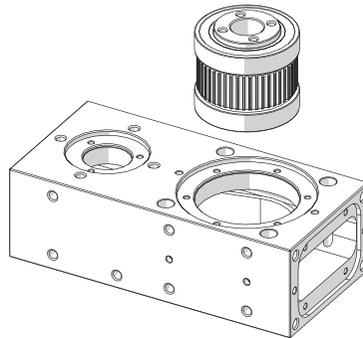
3. Insert the pinion assembly.
