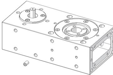
5. Rotate the tensioner anti-clockwise until the relevant notch points to the (-) mark.
