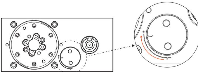
10. Check operation by rotating the rotaty flange for at least one turn, in both directions, applying to the pinion shaft the maximum torque shown in the table. The test is passed if the rotation is completed in both directions smoothly and evenly.
