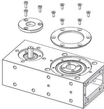
6. Install the rotary flange/s with the screws applying the tightening torque shown in the table. It is recommended to apply threadlocker like Loctite 243.
