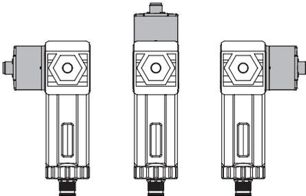
**N.B.:** If the FLUX is used downstream a Syntesi® filter, fit it in one of the three positions shown in the figure.
