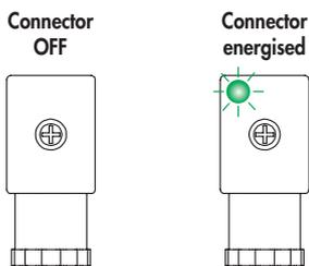
N.B.: For correct operation, both connector and coil need to be connected for the entire duty cycle (full power and reduced power); any electrical connection of the Energy-Saving connector to the coil during the reduced power phase **may cause the solenoid valve to be uncorrected switch**.
