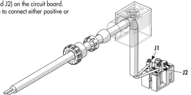
The connector circuit board has a green LED that comes on when the coil is energised.
